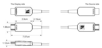
Figure 1: HDMI Connectors – SOURCE and DISPLAY (with Dimensions)
