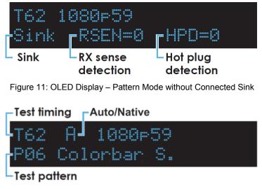
Figure 12: OLED Display – Pattern Mode with Connected Sink
