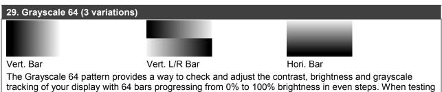
a display, no color should be visible in any of the bars, and all bars should be visible and distinct. There are 3 variations: 64 vertical bars, two sets of 64 vertical bars with the lower set reversed, and 64 horizontal bars.
