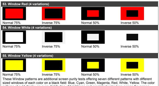
patterns should display an even distribution of brightness and consistent color tone across the screen. Each pattern has 4 variations: Normal 75% Window, Inverse 75% Window, Normal 50% Window, and Inverse 50% Window.
