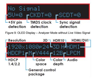
Figure 10: OLED Display – Analyzer Mode with Live Video Signal
