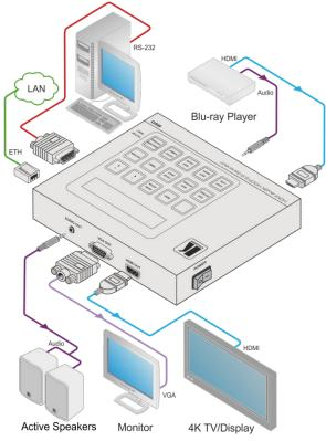
Figure 4: Connecting the 860 HDMI 18G Signal Generator & Analyzer
