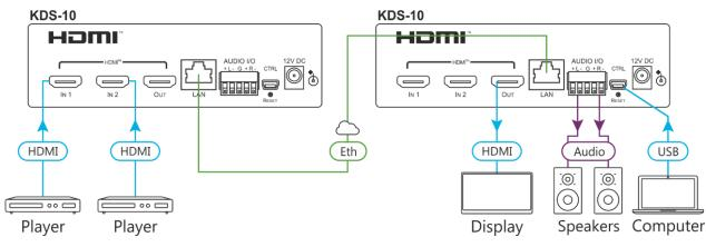
Figure 2: Connecting to the KDS-10 Rear Panel
