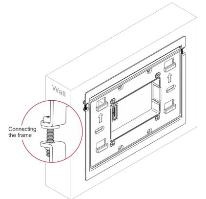
After hanging the KT-107 on the wall, tighten the two screws until the KT-107 is securely fixed in place.
