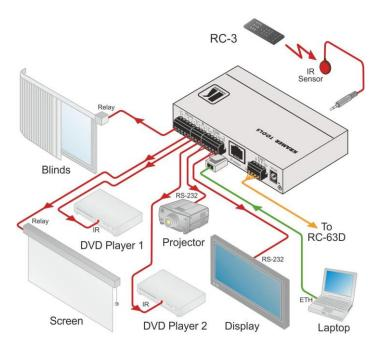
Figure 2: Connecting the SL-1N Master Room Controller
