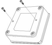
2. Fasten two screws to the bottom of VIA GO<sup>2</sup>.
