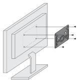
1. Attach the VESA mounting bracket to the back of the display with 4 screws.
