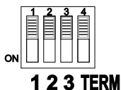
Figure 9: DIP-Switch Setup on a Single Machine
