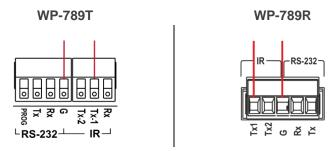
Figure 9: Connecting 38kHz IR Emitter - 38kHz
