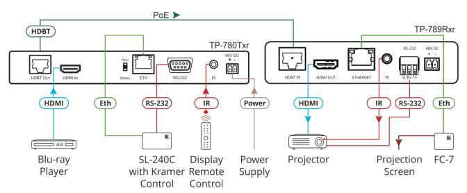
Figure 7: Connecting TP-789R/TP-789Rxr as PoE Acceptor
