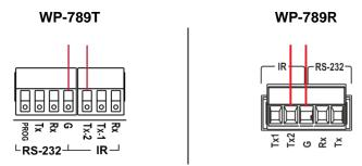
Figure 10: Connecting IR Emitter - Wide-Range Modulated
