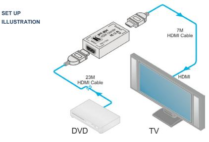
The **PT-2H** input is connected via a long male-to-male HDMI cable (not provided) to an HDMI source, such as a DVD player or a satellite set top box.
