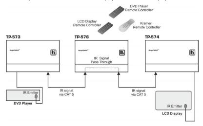
Figure 4: TP-576 IR Control - Example I
