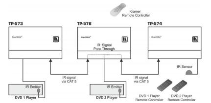
Figure 6: TP-576 IR Control - Example III
