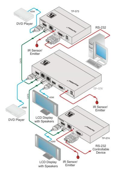
Figure 2: Connecting the TP-576 HDMI/CAT 5 Line Driver
