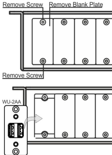
3. Reinsert the two screws to affix the wall plate insert in position, and tighten them.
