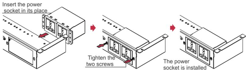
Figure 3: Installing the Power Socket
