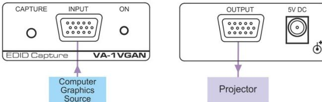
Always use Kramer high-performance cables for connecting AV equipment to the **VA-1VGAN**.
