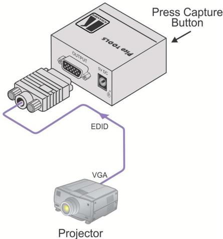
Figure 2: Acquiring the EDID from the Display Device
