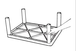
**1**Lay top shelf (with 4 leg posts only), ribbed side up on a smooth surface. Begin cart assembly by pushing 1 set of 4 legs onto leg posts.
