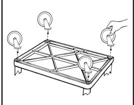
Push the four casters firmly into the holes in each corner of the bottom shelf (for big wheel models insert two 4" casters on narrow end of cart and follow big wheel instructions on next page). Important: casters must be fully seated. Tap firmly with rubber mallet to properly seat casters. Turn your Endura Linen Cart right side up, it is now ready for use.
