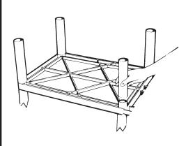
Place the next set of legs onto leg posts of shelf with handle and firmly hammer until properly seated. Repeat for all middle shelves.
