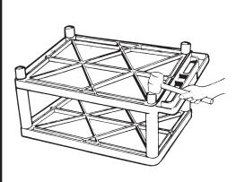
**2**Position second shelf over the 4 legs and insert leg posts into legs. Using a rubber mallet, firmly hammer shelf into legs until all four legs are seated (flush) against the surfaces of both shelves.
