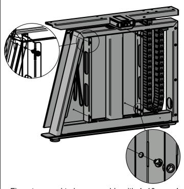
Fix outer panel to leg assembly with 4x10mm x4.
