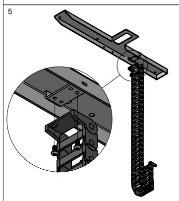
Fit energy chain to T plate using 10mm M6 button head fixings.
