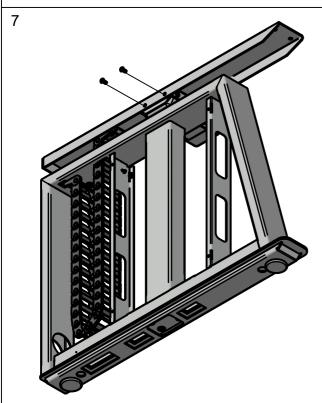
Fit T plate to bracket fitted to actuator using 10mm M6 button head fixings.
