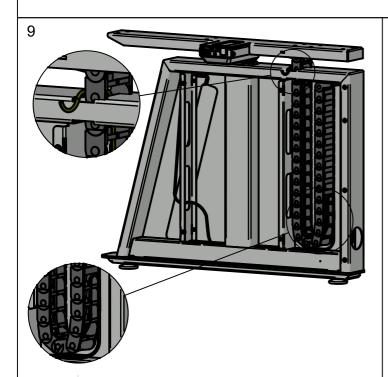
Feed cables all the way through leg frame, into the energy chain and out the top of the leg. see page 12 for further cable routing examples.
