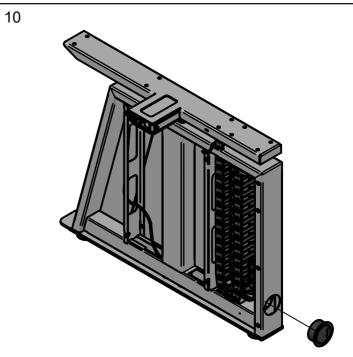
Fit cable cap to rear of leg assembly. Repeat steps 1 to 9 for opposite leg assembly.
