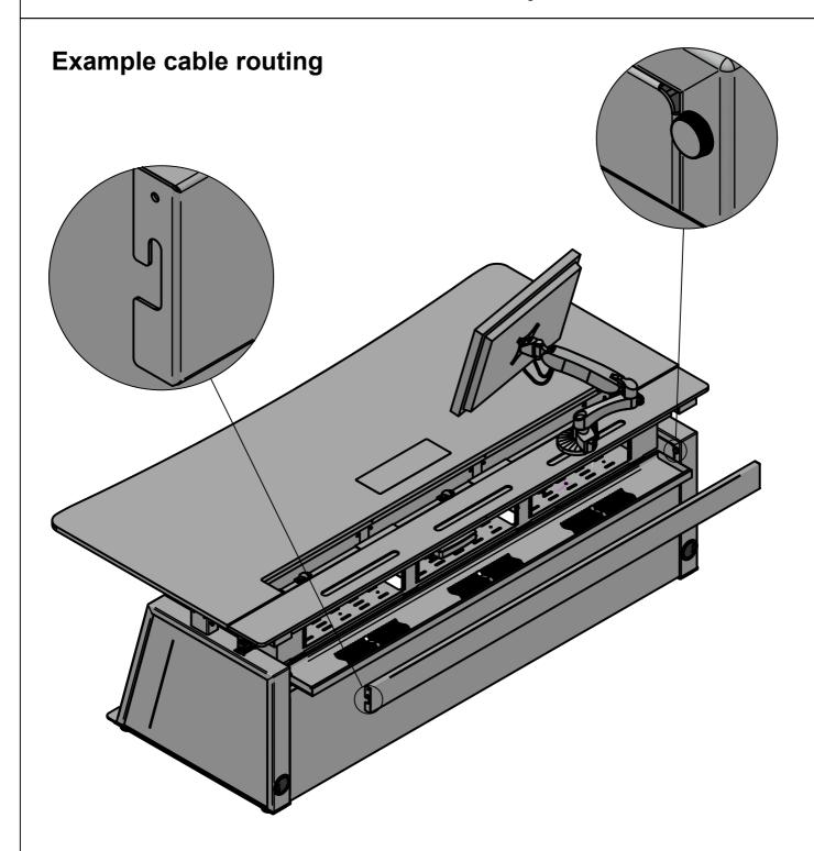
On fixed height desks and height adjustable desks in the lower position access to cable tray box rear door can be achieved by loosening thumbscrews and removing small modesty panel.
