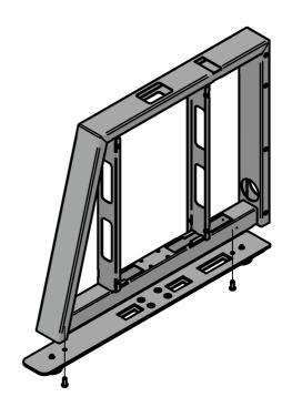
Fit foot plate to leg frame with 25mm M8 button head fixings.
