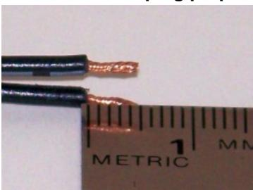
Unplug the power supply from the outlet first; cut off the original DC plug if using a non-Luxi power supply, separate the two wires for about 1" (2.5 cm) long, strip off the wire insulation precisely 3/16" (5 mm) from the end; too short a lead won't provide enough for the plug screws to catch; too long a lead may create short circuit). Identify the positive and negative leads; Luxi power supply has a white strip on the positive wire. If not sure, use a multi-meter to
