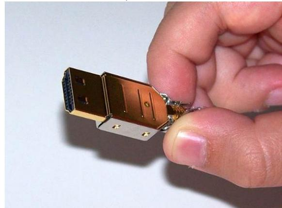
3.4 Slide the connector core into the top metal shell, push up with your thumbnail until you hear or feel a click
