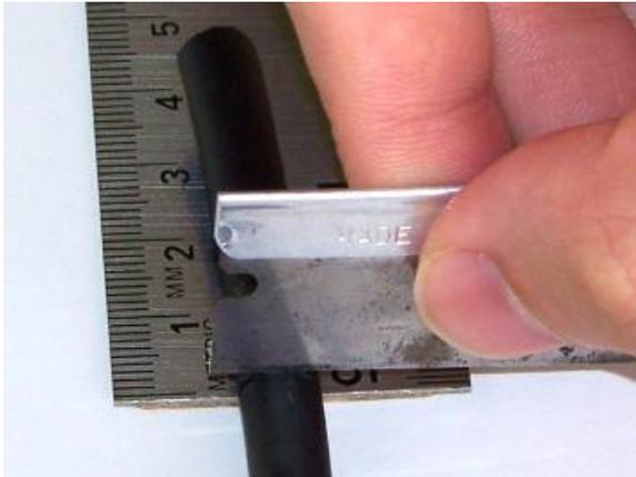
1.2 Use the blade to slice along the cable overall jacket then peel off the overall jacket
