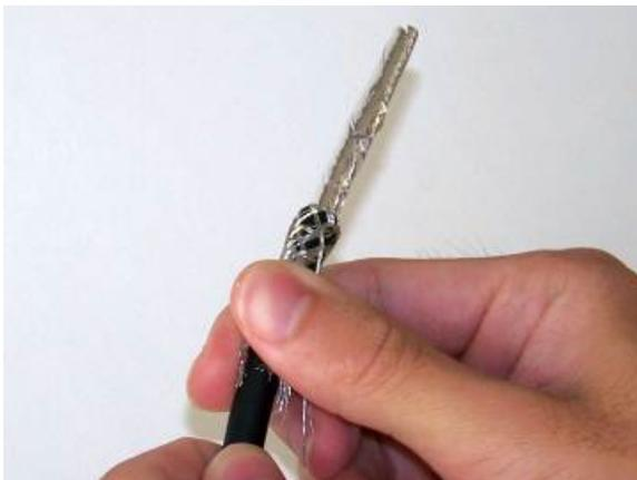
1.4 Remove the overall aluminum foil; now the 19 wires inside the HDMI cable are exposed
