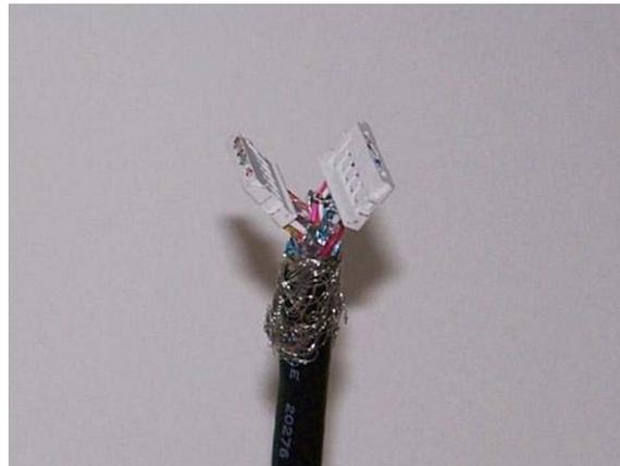
During the pre-crimp the recessed blade would cut off the wires and a tiny slice of the wire holder; this is normal.
