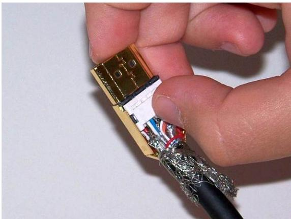
3.7 Use the hand tool's No. 3 dies to crimp the strain relief tabs onto the cable jacket with regular wires; make sure it's a tight crimp
