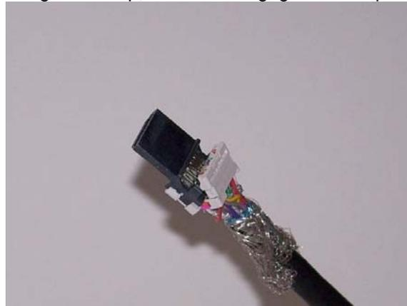
3.2 Use your fingers to press the wire holders into the connector core half way
