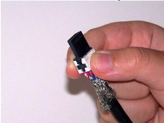
3.5 Place the bottom metal shell onto the top metal shell, line up the 4 notches, push together until you hear or feel clicks
