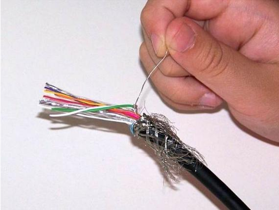
1.8 Fan the wires out into two groups based on color coding on page 1
