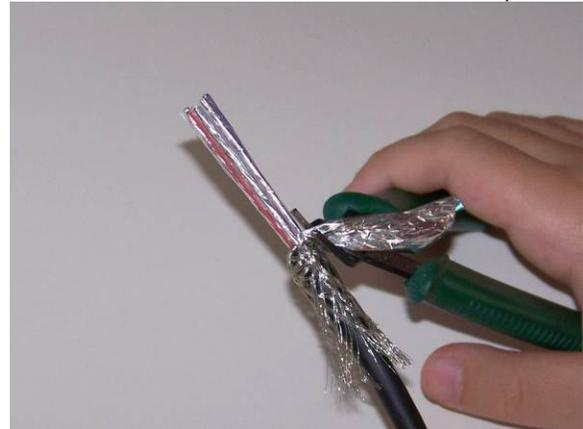
1.5 There are 4 twisted pairs. Cut off the plastic wrap on each pair 1/4" (6 mm) from the end
