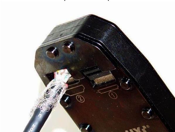
3.6 Use the finger tips to gently bend the strain relief tabs inward; be careful not to be cut
