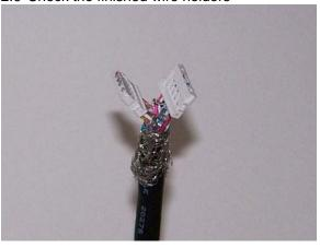
During the pre-crimp the recessed blade would cuts off the wires and a tiny slice of the wire holder; this is normal.
