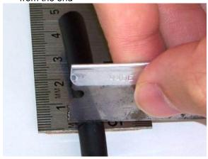
1.2 Use the blade to slice along the cable overall jacket then peel off the overall jacket
