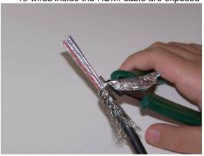
1.5 There are 4 twisted pairs. Cut off the plastic wrap on each pair 1/4" (6 mm) from the end
