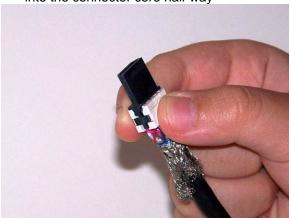
3.3 Insert the connector core with both wire holders all the way into No. 2 hole of the hand tool and perform crimp
