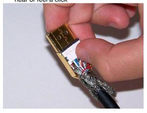
3.5 Place the bottom metal shell onto the top metal shell, line up the 4 notches, push together until you hear or feel clicks
