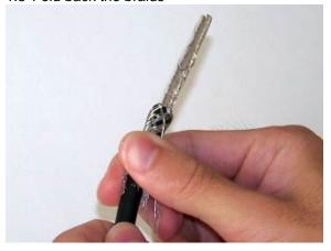
1.4 Remove the overall aluminum foil; now the 19 wires inside the HDMI cable are exposed
