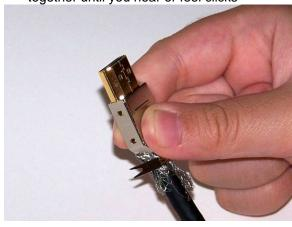
3.6 Use the finger tips to gently bend the strain relief tabs inward; be careful not to be cut
