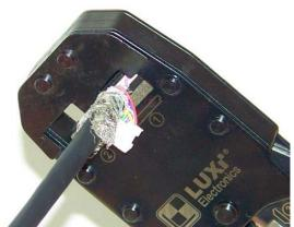
2.5 This tool has a ratchet design. If you ever need to release the latch, turn the thumb nail in the marked direction
