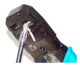
2.4 Slide and line up the other wire holder to about the same position; repeat the precrimp to it. <u>Inspect the wire ends for any</u> potential short
