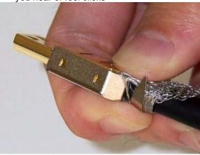
3.5 Use the finger tips to gently bend the strain relief tabs inward; be careful not to be cut
