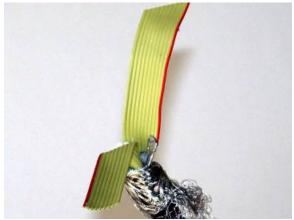
Note: The newer ribbon wires changed the red stripes to black and wire stripes, for easy matching with black and white wire holders, respectively.
