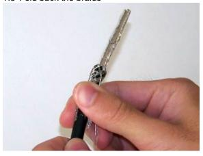
1.4 Remove the overall aluminum foil; now the 2 ribbons inside the HDMI cable are exposed
