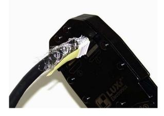
2.6 During the pre-crimp a recessed blade would cuts off the wires and a tiny slice of the wire holder; this is normal
