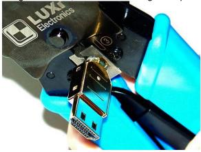
3.7 Trim off the excessive drain wires
