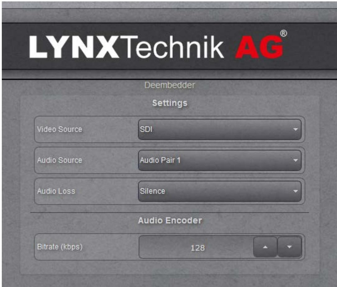
An additional setting is available to configure the behavior on loss of input. The selection for this parameter is "Off", "Silence" or "1kHz Test Tone".
