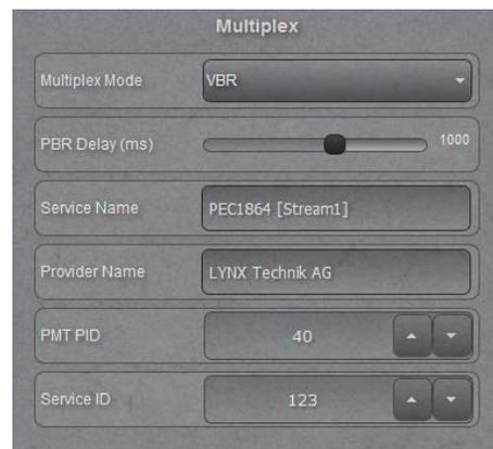
**Note:** *CBR: Constant Bitrate; VBR: Variable Bitrate; RVBR: Restricted Variable Bitrate (limited upper bandwidth; PBR: Policy Based Routing; PMT: Program Map Table*
