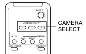
Then, you can operate the camera(s) specified by number. Every time you operate the camera(s) using the infrared remote controller, the CAMERA SELECT button pressed in step 2 lights.
