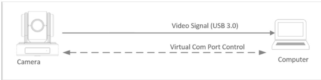
Before you use the virtual COM port, you need to install the driver onto your PC/Mac. You can download the driver (PL2303 Prolific Driver Installer v1.12.0) here: <http://plugable.com/drivers/prolific>
