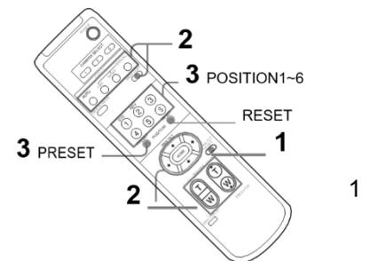
While holding down the PRESET button, press any of the POSITION buttons, 1 to 6, in which you want to store the settings.
