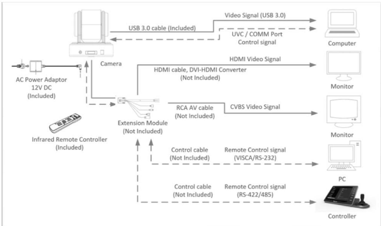
In this connection configuration, Extension Module, DVI-HDMI converter, DVI cable, HDMI cable, Analog video cable, data cable is required. To obtain these third party components or accessories, consult the dealer where you bought your camera.
