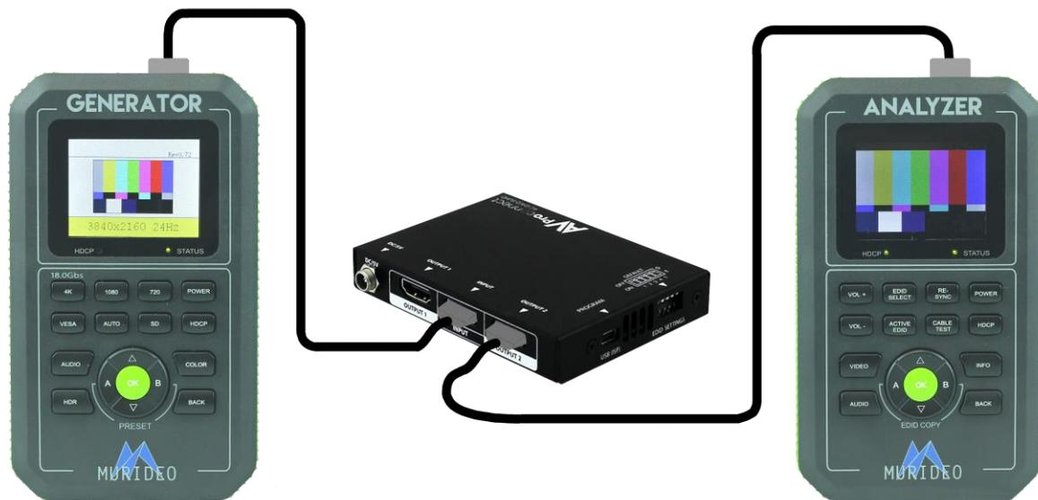
How to Test a Repeater (a repeater is any HDMI device that receives an input signal and retransmits that same signal to a downstream sink or display device; like a matrix, a switch, an AV receiver or distribution amplifier)
