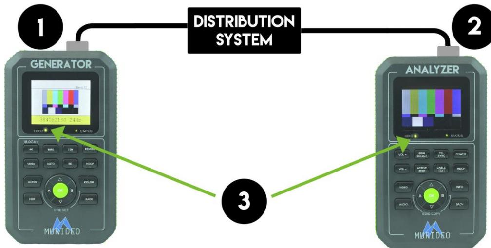
In the system diagram above it's easy to see the basic components of a video distribution system. Obviously, this is a very simple system diagram, use your imagination to replace all the sources, displays, matrices, distribution amplifiers and extenders in the system [where you see the term – DISTRIBUTION SYSTEM above] and the task of troubleshooting these systems can become daunting at times.
