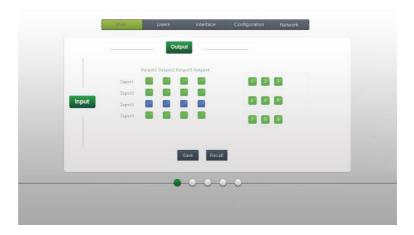
The matrix grid displays all possible connections between each input and output. Users can make connections by clicking on the corresponding grid button.
