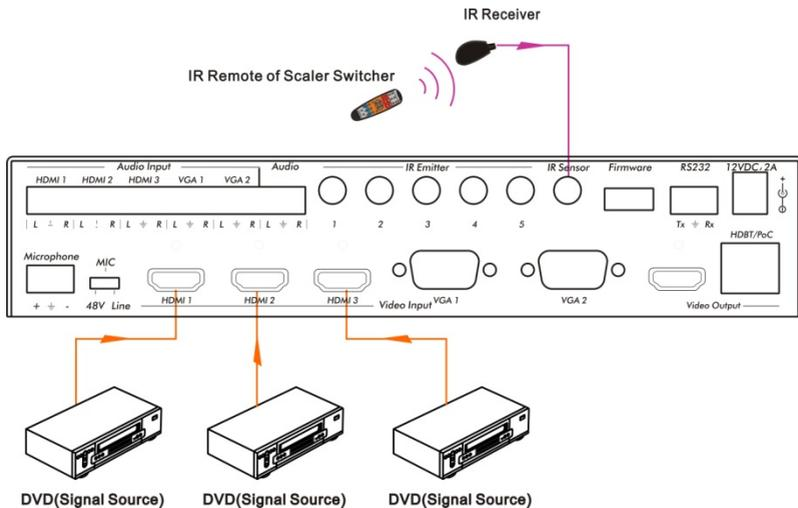
**CEC: Control HDMI source devices by IR remote**
