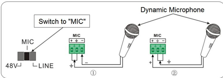
**2) Balanced connection:** “+” connects to positive, “-” connects to negative and “ $\text{---}$ ” connects to ground.
