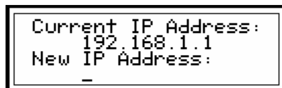
Figure 16- Set IP Address from LCD and keypad
