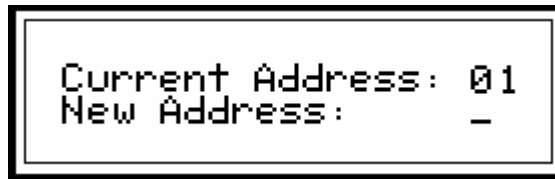
Figure 14- Set Serial Address from LCD and keypad
