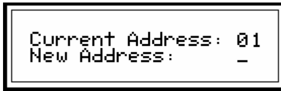
Figure 14- Set Serial Address from LCD and keypad
