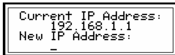
Figure 16- Set IP Address from LCD and keypad
