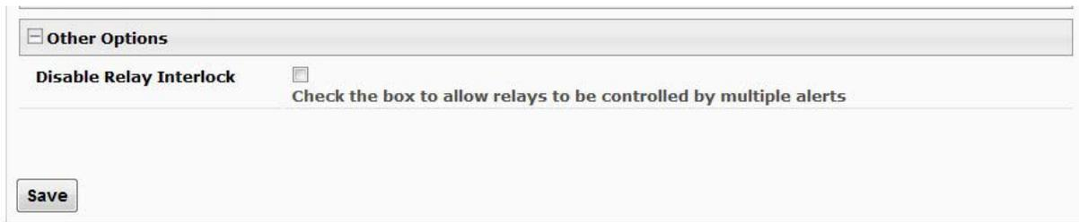
Figure 70- Disable/Enable Relay Interlock
