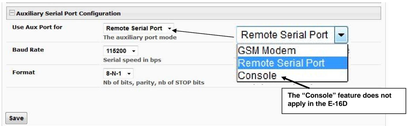
Figure 67- Configure the purpose of the "RS232 AUX" port
