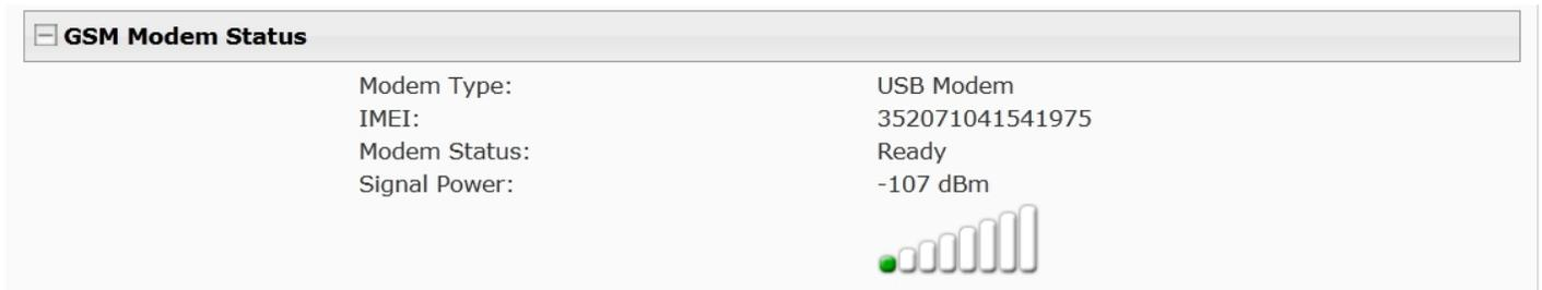
**Modem properly installed in an E-xD (Note: Signal strength shown here is extremely poor)**
