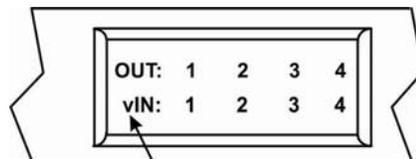
LCD WILL CYCLE TO DISPLAY A “v” FOR ALL VIDEO INPUTS FIRST, THEN A “a” FOR ALL AUDIO INPUTS.
