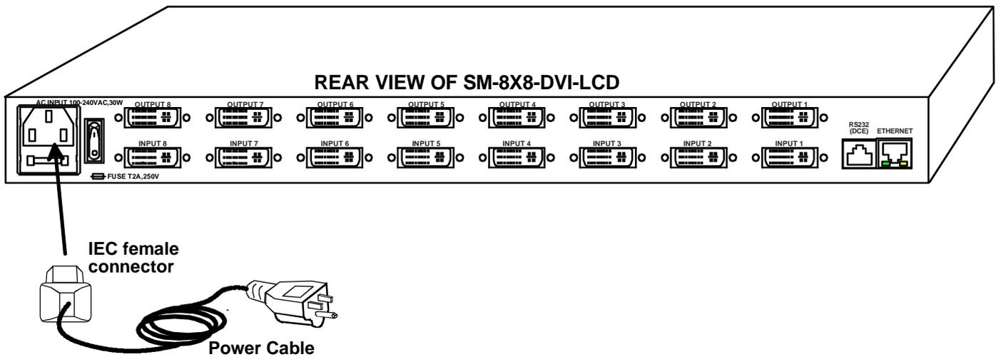
**Figure 8- Attach AC power cord to VEEMUX**
