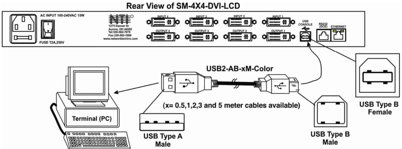
Figure 6- Connect RS232 using USB cable
