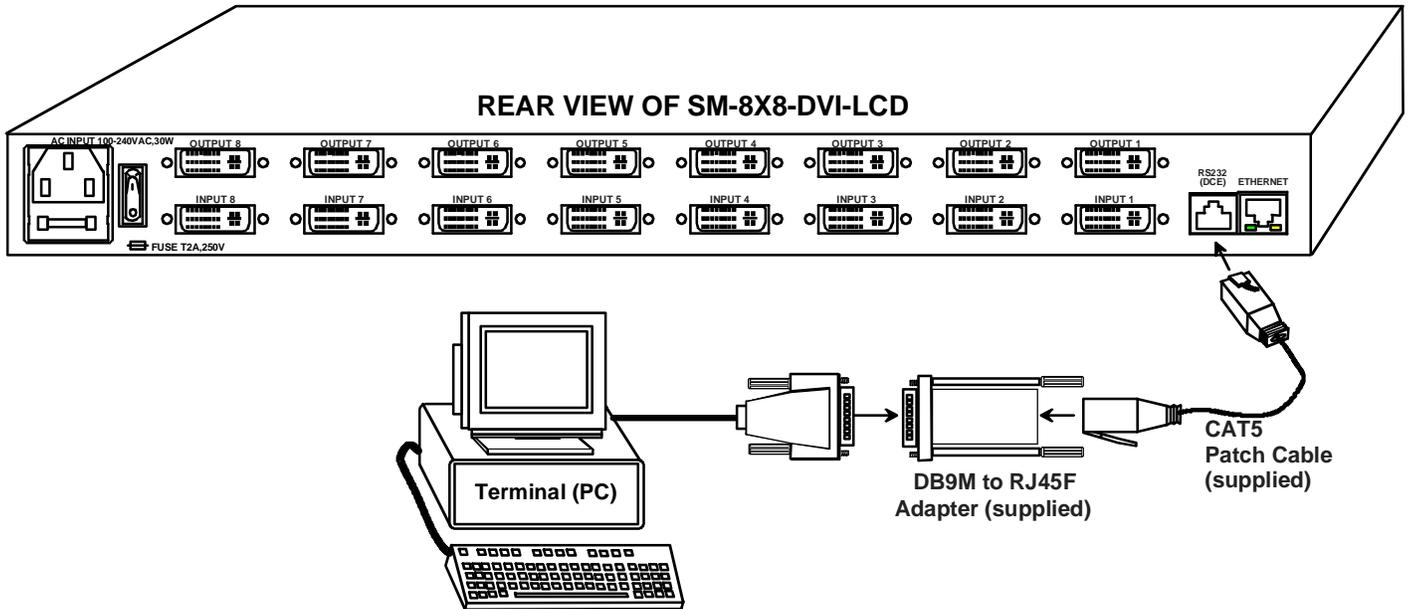
Figure 5- Connect RS232 control terminal to VEEMUX
