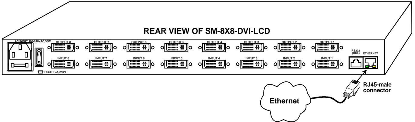
**Figure 7- Connect VEEMUX to local area network**
