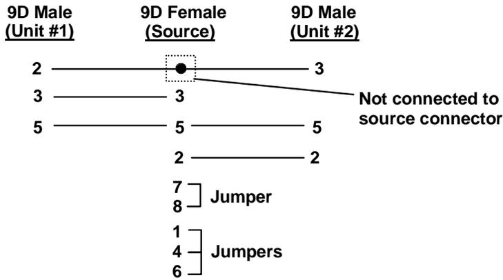
Figure 13- Pinout of Matrix-Y-1 cable
