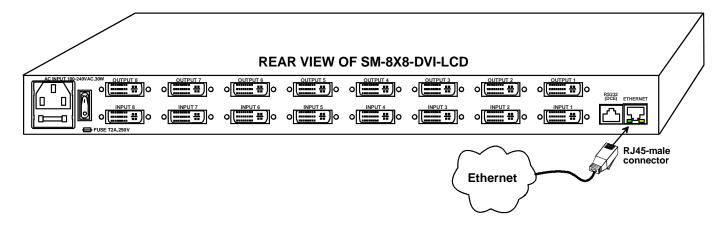
Figure 7- Connect VEEMUX to local area network
