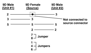
Figure 13- Pinout of Matrix-Y-1 cable
