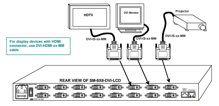
Figure 4- Connect display devices to VEEMUX
