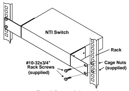
Figure 2- Secure switch to a rack
