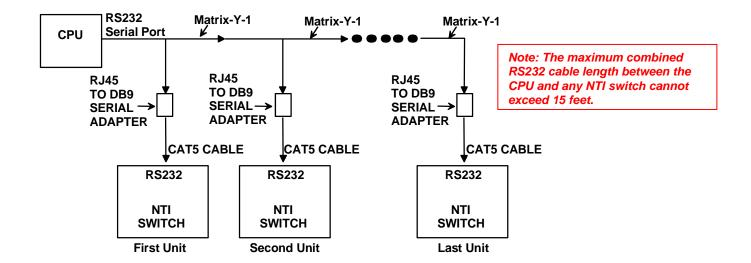
Figure 12- RS232 connection with Matrix-Y-1 cable
