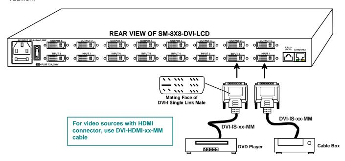
Figure 3- Connect video sources to VEEMUX
