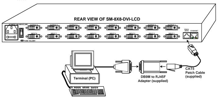
Figure 5- Connect RS232 control terminal to VEEMUX
