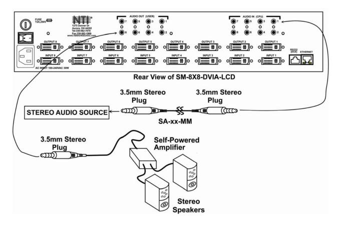
Figure 9- Connect Audio Source and Speakers
