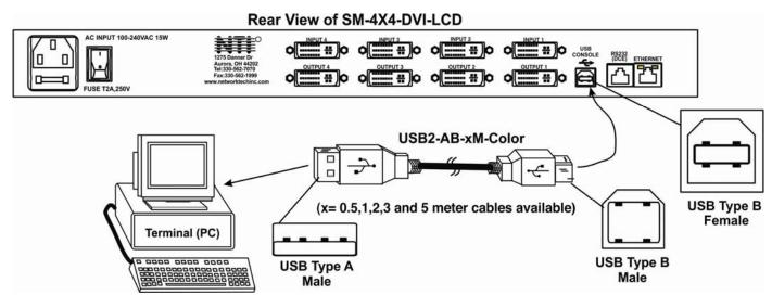
Figure 6- Connect RS232 using USB cable
