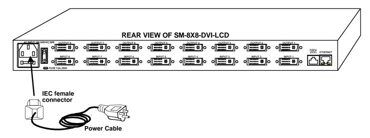
Figure 8- Attach AC power cord to VEEMUX
