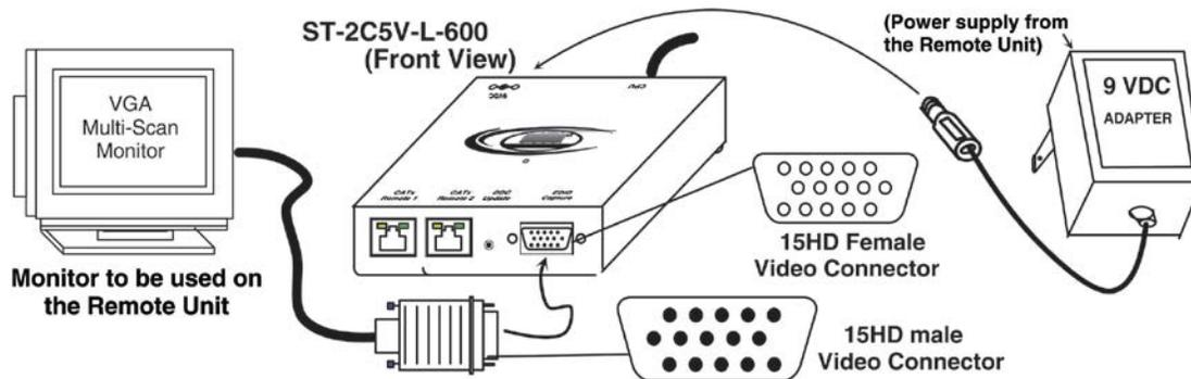
Figure 25- Connect remote monitor for EDID capture
