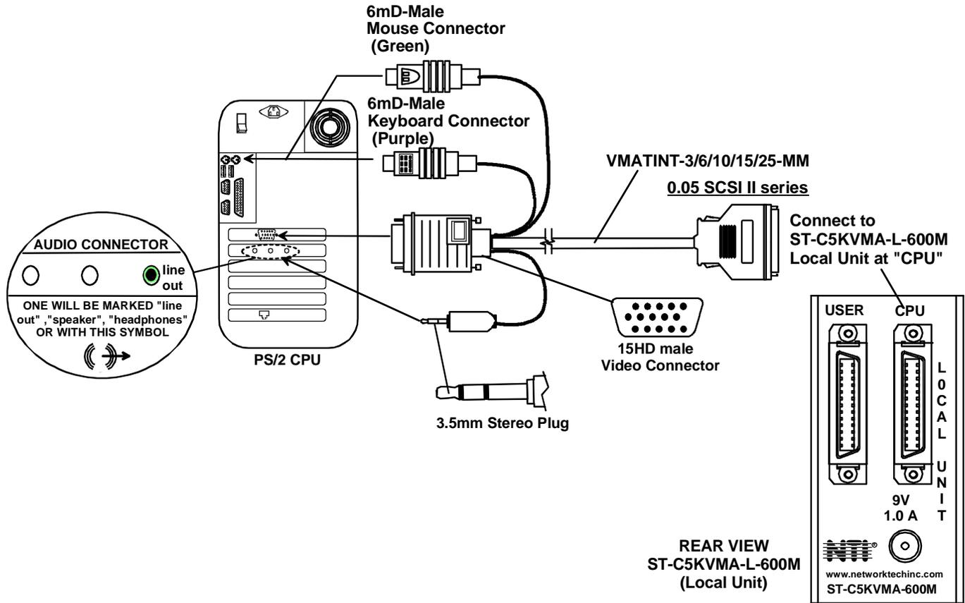
Figure 19- Connect cable between CPU and module
