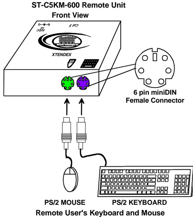
Figure 12- Connect keyboard and mouse to Remote Unit
