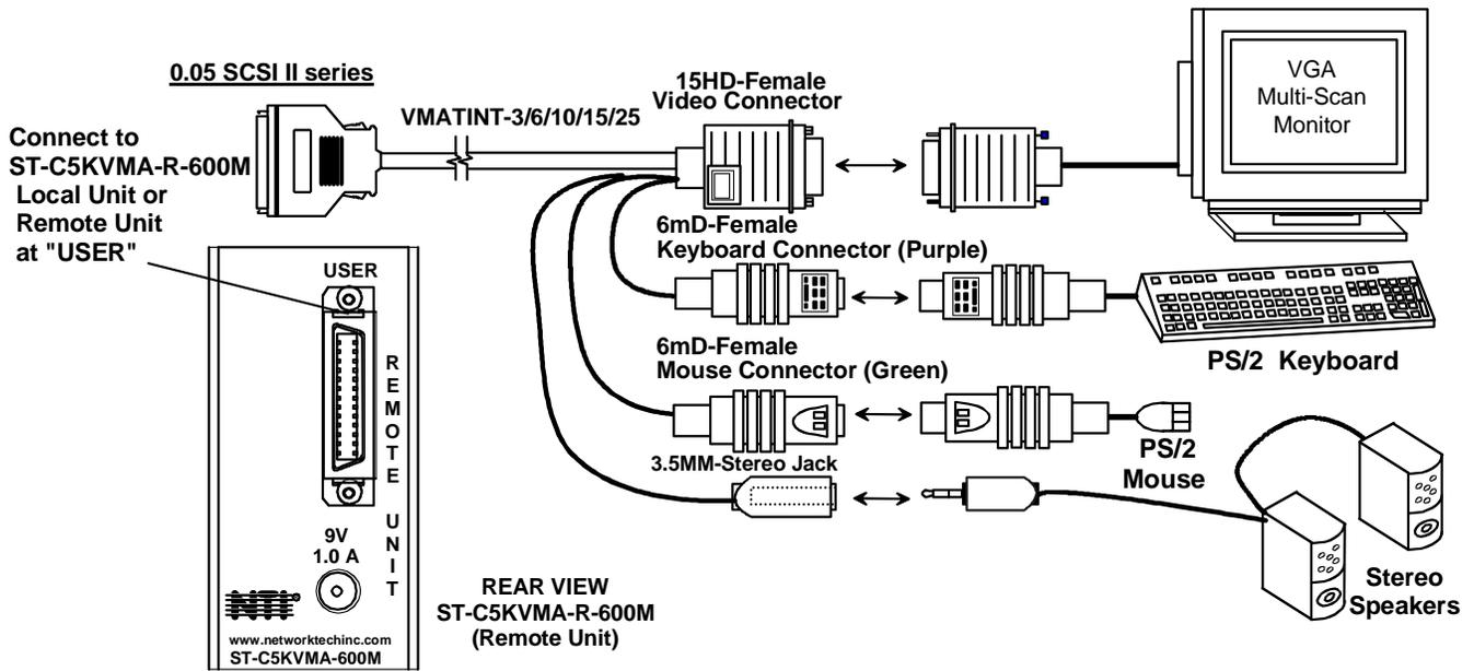
Figure 20- Connect cable between user and module
