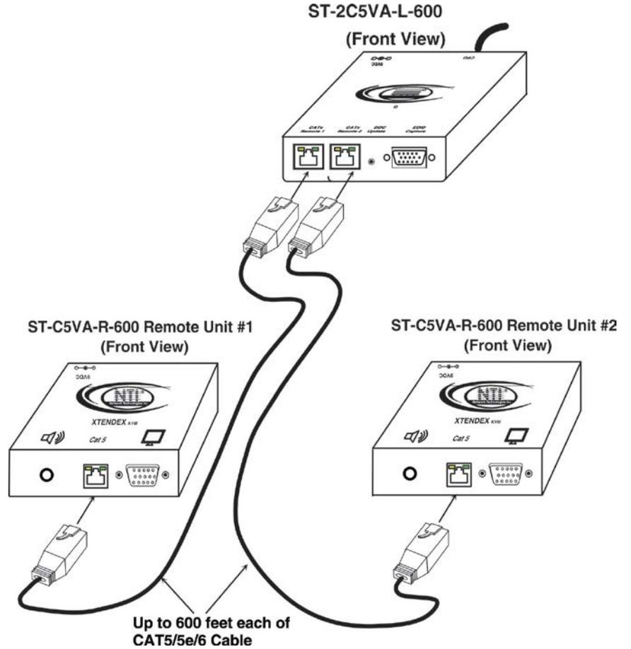
Figure 14- Connect CATx cables between Local and Remote Units
