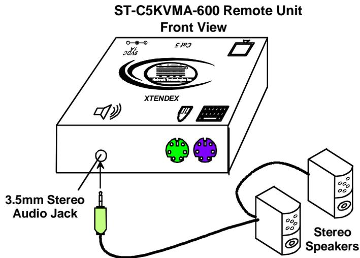
Figure 10- Connect speakers to the Remote Unit
