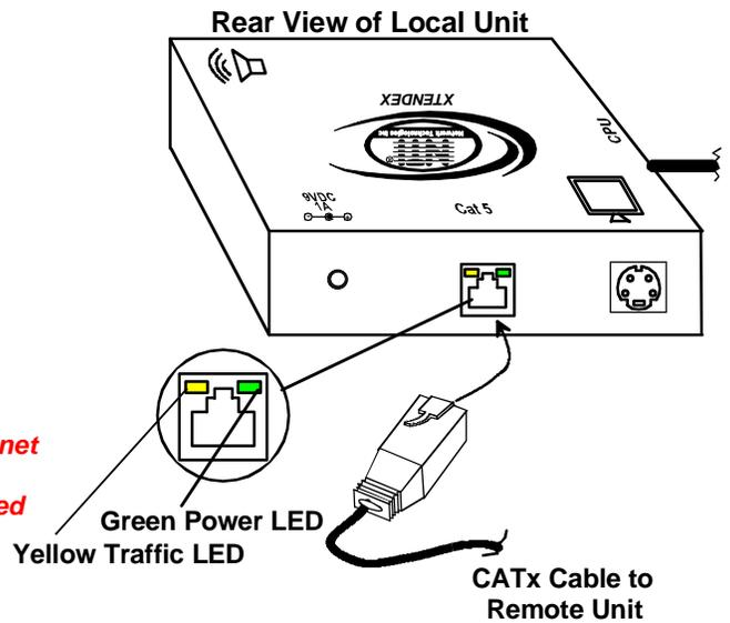
Figure 8- Connect CATx cable to Local Unit
