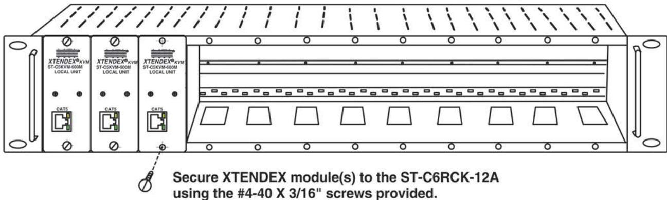
**Figure 17- Secure each module to the tray**
