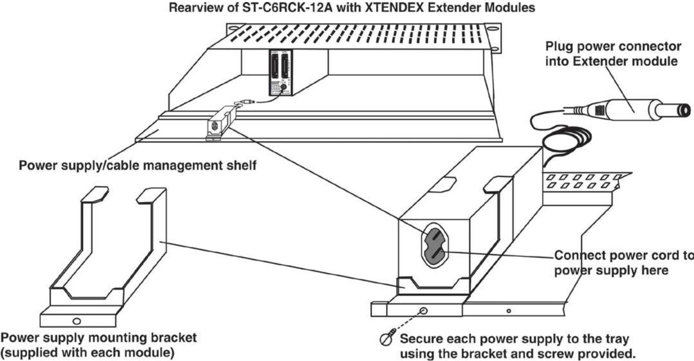
Figure 18- Secure each power supply to the tray
