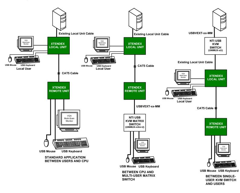
Figure 7- Examples of common applications
