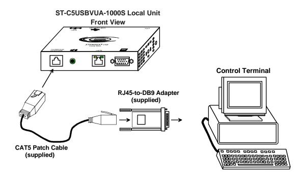
Figure 8- Connect PC for firmware upgrade
