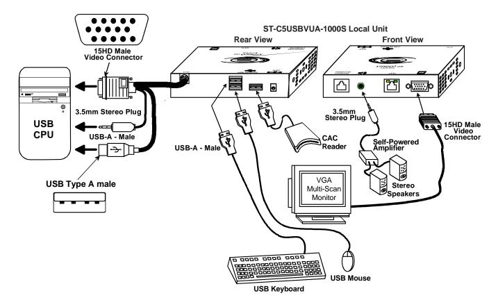
Figure 1- Connect the Local Unit to a CPU
