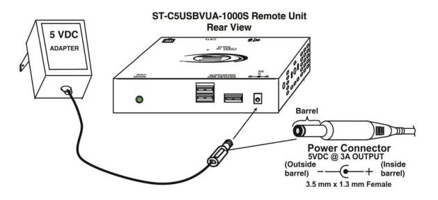
Figure 5- Connect AC adapter to Remote Unit
