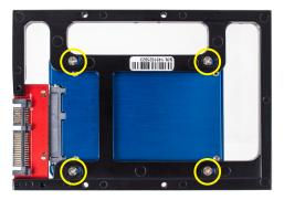
Once the screws are fastened the top view should look like the photo below. The AdaptaDrive can now be integrated with your desktop computer or drive enclosure.
