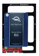
Insert the AdaptaDrive into the computer or enclosure of your choice. Four additional screws are included, but you may find that your computer or enclosure already includes screws or other mounting components. The NewerTech AdaptaDrive can be installed into your computer's 3.5 inch SATA drive bays as well. The example below shows the AdaptaDrive being installed into a Mac Pro.
