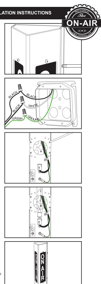
REMOVE THE 4 FLAT HEAD PHILLIPS SCREWS FROM THE TOP OF THE HOUSING AND SET THEM ASIDE. SEPARATE THE HOUSING FROM THE BACK PLATE AND REMOVE THE WIRE NUTS AND SCREWS THAT ARE INSIDE.
