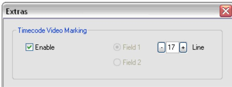
Timecode stamping must be enabled in the driver before it can be used, and the field and line number correctly set. The Osprey 530/540/560, unlike the Osprey 100 and 200 series devices, does not implement an autosearch function to find the VITC line. To access the controls, go to the Device property tab and click **Extras...**
