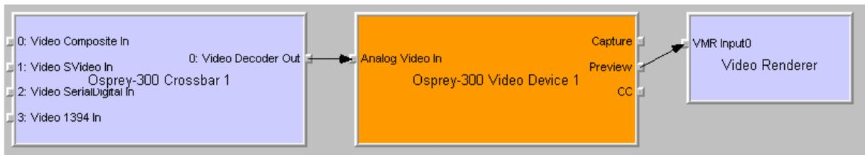
VMR7 is short for Video Mixing Renderer 7. VMR7 is a newer renderer that is generally much faster than the old Video Renderer. When the driver is running in Direct Mode, VMR7 uses an efficient DirectDraw configuration to render with almost no CPU overhead, especially when YUY2 video is used. When the driver is running in PostProcessing Mode, DirectDraw is not used but it is still the fastest renderer.
