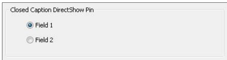
This group controls whether the closed caption (Figure 40) character pairs emitted by the DirectShow closed caption pin are from field 1 or field 2 of the video. The DirectShow specification is that closed caption on a closed caption pin is always from field 1; however, this extension allows application developers to access field 2 data such as XDS data (including Vchip) via a DirectShow standard pin.
