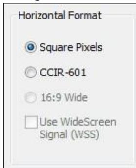
**Square Pixels** - This setting is for normal 4:3 video that will be viewed via a computer monitor. This setting results in a square aspect ratio sampling of the source video and a source image of 640 x 480 for 525-line standards and 768 x 576 for 625-line standards.
