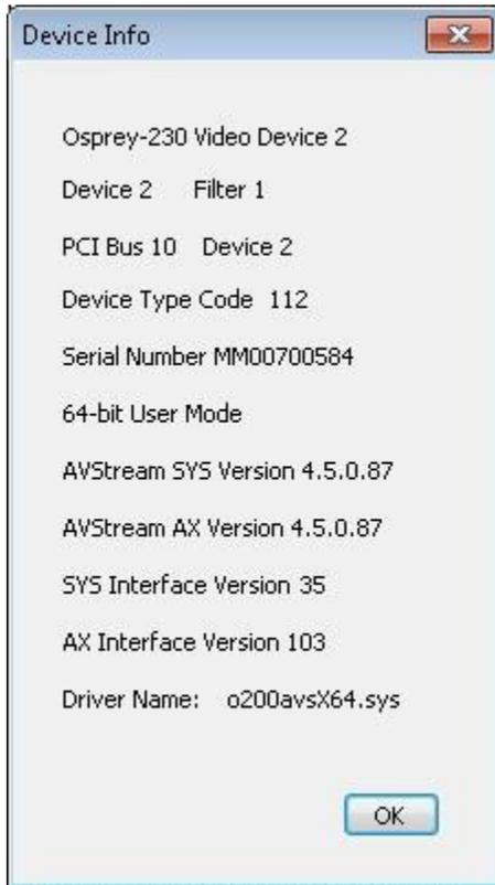
This button displays useful information about the capture card and the driver, including the DirectShow name of the device (Figure 36).
