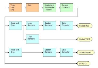
Figure 53 shows a possible graph of video data flow within the driver in PostProcessing Mode. This particular graph assumes that SimulStream is activated so that more than two video pins are possible. There are four video output pins, represented by the pale yellow round rectangles:
