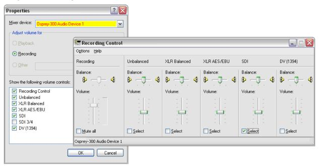
To get to the Osprey audio capture (recording) device, select Properties under Recording Control's Options menu. This pops up the Properties dialog. Click on the Mixer device list at the top to see the list of audio input and output devices, including one or more Osprey cards. When you have chosen the device, click **OK**, and you will be returned to the Recording Control display.
