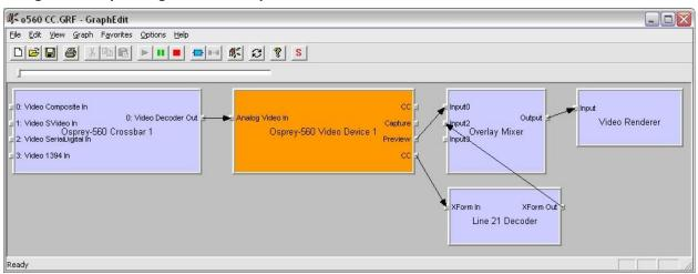
The driver supports the standard DirectShow CC and VBI pins (on the Osprey 530/540/560, the CC pin only; on the other products, both pin types). The CC character pair data can be streamed to applications such as Windows Media Encoder 9, or rendered directly to the screen using the DShow Overlay Mixer filter. The 4.0.0 driver can be set to output CC field 2 character pairs on the CC pin, instead of the standard CC field 1 data. XDS (Vchip) data is embedded in the field 2 stream.
