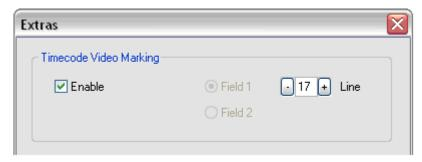
Timecode stamping must be enabled in the driver before it can be used, and the field and line number correctly set. The Osprey 530/540/560, unlike the Osprey 100 and 200 series devices, does not implement an autosearch function to find the VITC line. To access the controls, go to the Device property tab and click **Extras...**
