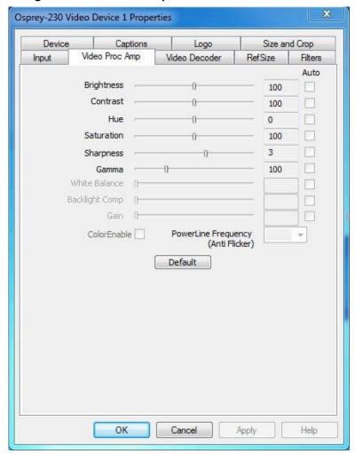
Slider controls let you adjust brightness, contrast, hue, saturation, sharpness and gamma. If you're using the preview or capture mode in real-time, then you can see your adjustments as you make them with the Video Proc Amp controls. If preview or capture-to-screen video is running when you access this page, you can see your adjustments interactively.
