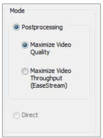
The Mode group (Figure 27) selects the two main functional modes of the driver – PostProcessing Mode and Direct Mode – as well as the Quality/Throughput tradeoff for PostProcessing Mode.
