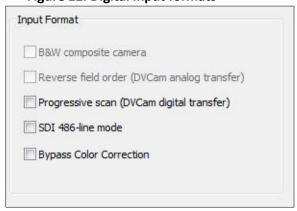
When a digital input (SDI or DV (1394)) is selected, the analog controls are grayed and three controls relevant to digital inputs are enabled.
