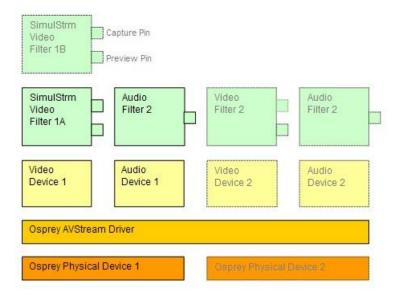
At the bottom of this diagram are one or more physical Osprey hardware devices. All Osprey devices of a given type (such as Osprey 230 or Osprey 560) are controlled by a single Osprey binary, the Osprey AVStream Driver. For each physical device the AVStream Driver creates one logical Video Device and one logical Audio Device.
