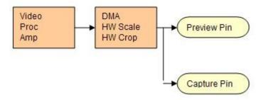
The purpose of Direct Mode is to capture and/or preview video with very low CPU overhead. It is meant for low capability machines and for other cases where it is imperative for the driver to use as little CPU as possible. Scaling, cropping, and color conversion are done in hardware, incurring no processing overhead – but at the cost of reduced flexibility.
