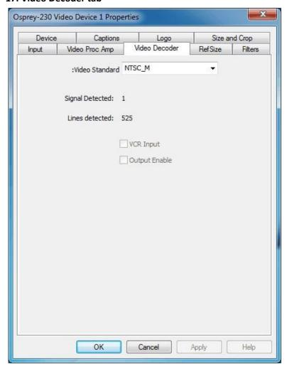
Changes apply to all video previews and stream captures on the currently selected device. If you have multiple Osprey cards, you can set the input individually for each of them. Changes made with this control take effect immediately. If video is running and a standard is selected that does not match the incoming signal, the video is likely to freeze or glitch until the signal matches the correct standard.
