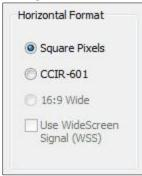
**Square Pixels** - This setting is for normal 4:3 video that will be viewed via a computer monitor. This setting results in a square aspect ratio sampling of the source video and a source image of  $640 \times 480$  for 525-line standards and  $768 \times 576$  for 625-line standards.
