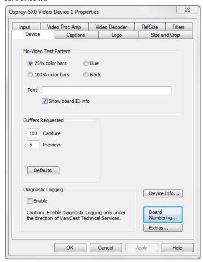
The Device tab has the following controls.
