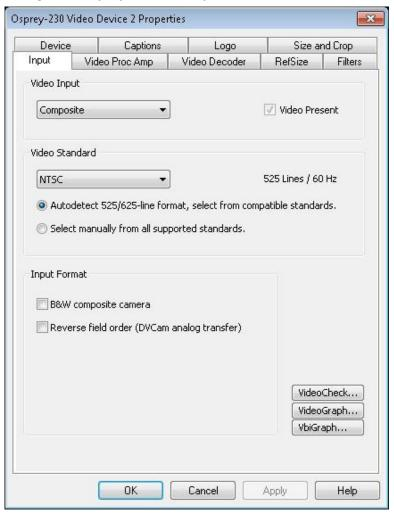
Figure 5. Osprey's Device Properties window
