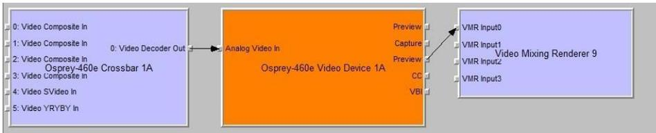
Video Mixing Renderer 9 is the newest video rendering method and the one on which Microsoft supposedly is basing its future development. The intent is to combine the functionality of the Overlay Mixer plus Video Renderer in one module that takes advantage of the latest developments in
