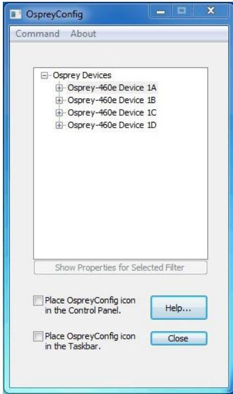
In this example, the computer in use has one card and four devices. The card can take a single input and stream the content differently, for example, you can use several bit rates, sizes, and formats.
