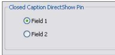
The Closed Caption DirectShow Pin (Figure 76) controls whether the closed caption character pairs emitted by the DirectShow CC pin are from **Field 1** or **Field 2** of the video. The DirectShow specification is that CC on a CC pin is always from Field 1; however, this extension allows application developers to access Field 2 data such as XDS data (including V-chip) via a standard DirectShow CC pin.
