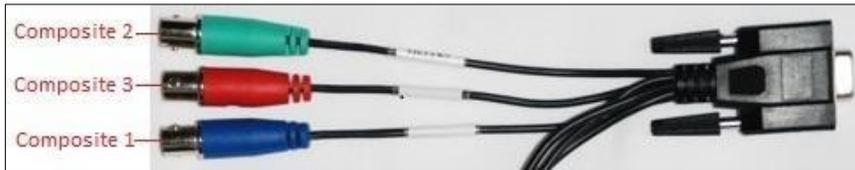
Finally, with an additional adapter, a SVideo source can be connected to this dongle. The SVideo connection replaces Composites 2 and 3, but Composite 1 is still available as shown in Figure 22.
