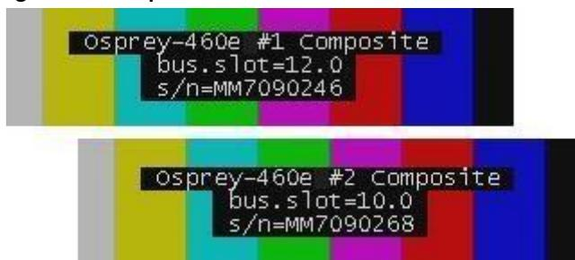
To set up the test patterns, enable the board ID information display by enabling **Show board ID** info on the Device tab (Figure 69).
