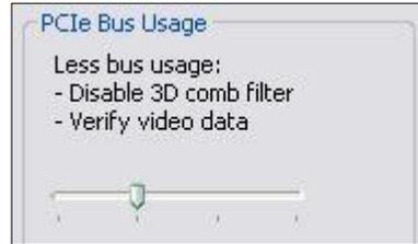
The rightmost position (Figure 56 and Figure 57) is for systems with high PCIe bandwidth, and especially for PCIe 2.0 systems. It disables video data verification and EaseStream and turns on 3D filtering. The warning message only appears for Osprey 260e/460e boards and should not discourage you from trying this setting, but ensures you understand that problems are likely on PCIe 1.X systems when multiple video streams are run.
