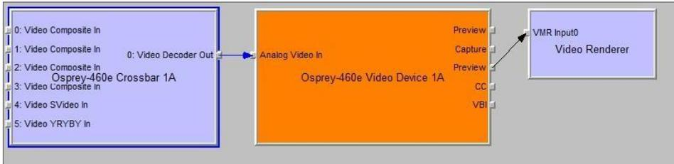
VMR7 is short for Video Mixing Renderer 7. VMR7 is a newer renderer that is generally much faster than the old Video Renderer. When the driver is running in Direct Mode, VMR7 uses an efficient DirectDraw configuration to render with almost no CPU overhead, especially when YUY2 video is used. When the driver is running in PostProcessing Mode, DirectDraw is not used but it is still the fastest renderer.
