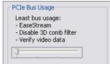
The third position (Figure 54 and Figure 55) disables 3D comb filtering and turns on video data verification, but turns off EaseStream. We have not seen any need for this setting yet in the systems we have tested so far. Use this setting when intermittent horizontal streaks appear in the video, especially when a lot of video streams are running.
