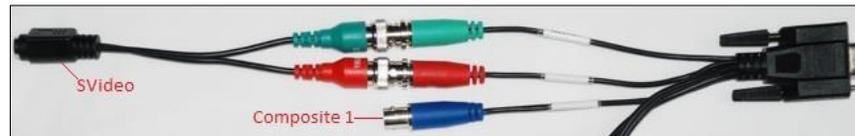
You can also use a Composite/SVideo dongle with the Osprey 210e, the connections are shown in Figure 23.
