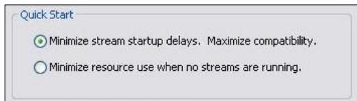
The Quick Start option also causes the first audio buffer and video frame to be delivered at close to the same time. This fact is important to some applications. Most mainstream applications determine correct sync from timestamps, and are therefore immune to differences between audio and video startup times. But some applications do not do this correctly, and for correct initial A/V sync the Quick Start option must be enabled.
