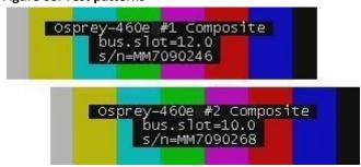
To set up the test patterns, enable the board ID information display by enabling **Show board ID** info on the Device tab (Figure 69).
