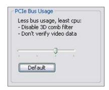
The Osprey Analog PCIe series driver uses three methods to ensure adequate PCIe bandwidth and prevent video data errors:
