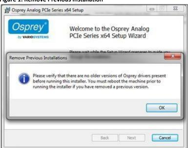
Figure 1. Remove Previous Installation
