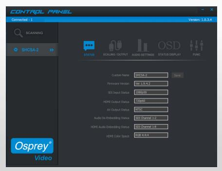
The Control Panel Software exposes additional features which are not accessible by the DIP Switches. It also allows the user to create custom settings and profiles which can be saved and later accessed by DIP Switch.
