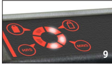
(9) A single button-press, whether the battery is on or off-load, displays charge status in terms of percentage. When batteries are linked this figure still relates to the battery's individual capacity. The lights indicate remaining capacity in percentage blocks:
