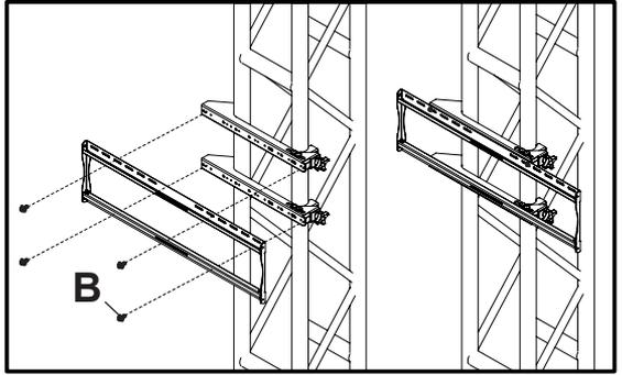
Use the outermost compatible hole positions to mount the plate supplied with separate mount and secure using taplite screws provided.
