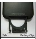
Push the tab, located on the left of the battery clip, to the right and pull out the clip.
