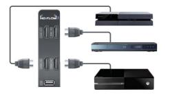
Connect HDMI cable from the Transmitter's passthru output port to the input of the display device to enjoy the video coming through HDMI1 only.
