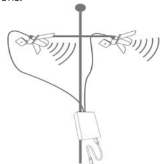
Pairs of Directional Antennas must be aimed to cover the same area.
