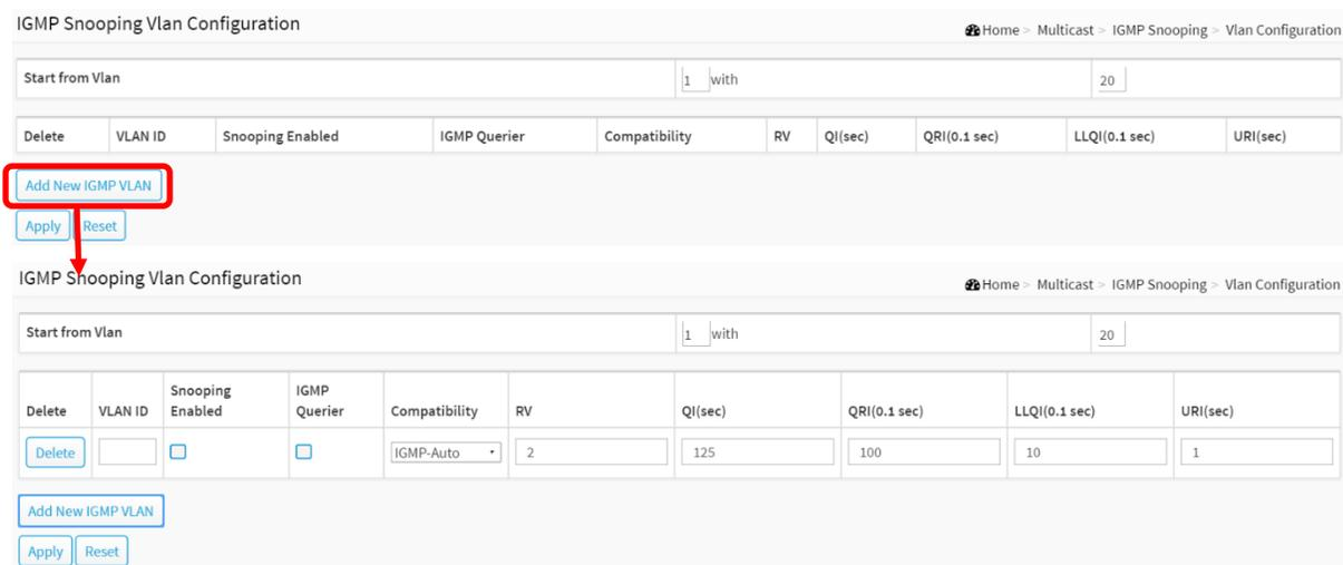
The screenshot shows two instances of the 'IGMP Snooping Vlan Configuration' web interface. The top instance shows the 'Add New IGMP VLAN' button highlighted with a red box and a red arrow pointing to the bottom instance. In the bottom instance, a new entry has been added to the table.
