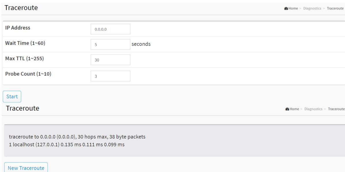
The screenshot shows two instances of the Traceroute web interface. The top instance is the configuration page with the following fields:
