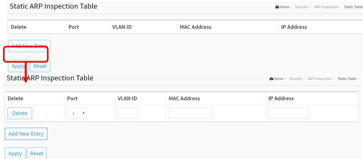
Figure11-4.3: The Static ARP Inspection Table
