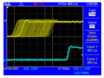
The cleaned and jitter-freed signal can be used as reference clock for any application, without any problem. The signal processed by SteadyClock is of course not only used internally, but also available at the ADI-6432's word clock output. It is also used to clock the digital outputs MADI and AES/EBU.
