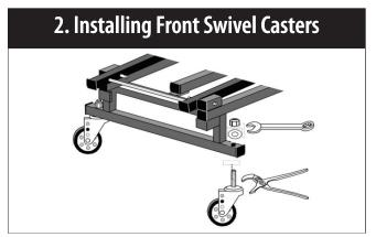
Carefully insert caster stem into receptor tube and line up caster stem holes with the receptor tube holes. Stem should fit very snugly in receptor tube. Install cotter pins and bend ends outward.
