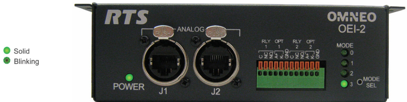
FIGURE 15. Single Keypanel – Channel 2 (LED 3 is solid)
