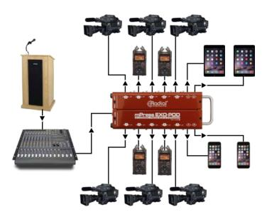
The optional mPress is a modular press box and command center that can be used on its own or with several Exo-Pod units to expand up to 448 outputs. Visit our website www.radialeng.com for more information on the mPress.
