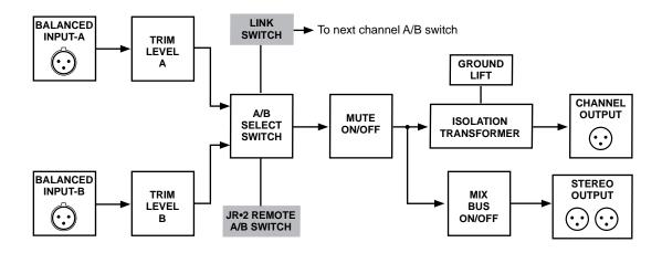
To eliminate hum and buzz caused by ground loops, each channel output is transformer isolated and equipped with a ground lift switch. These are rated to handle signal levels in excess of +20dB from 20Hz to 20kHz and work equally well when switching the outputs from professional mixing consoles as they do for wireless microphones and instrument level signals.
