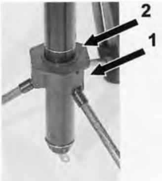
Loosen the central locking of the legs by pulling up the center plate **1** to the marker **2** at the center column.
