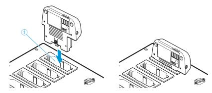
The charging process starts automatically (see "Behavior of the ADN-W BA battery pack during charging" on page 5). The status display ④ indicates the charging process (see "The status display of the ADN-W L 10 charger during charging" on page 4).
