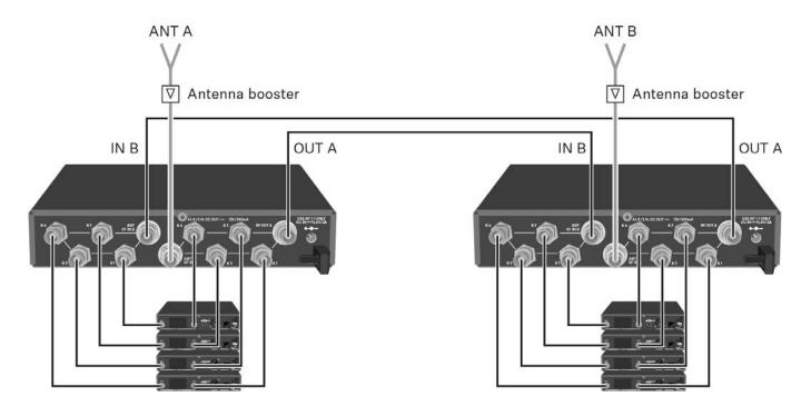
Option 3: Two antennas supply a 8-channel system
