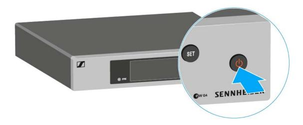
To switch the receiver to standby mode:
